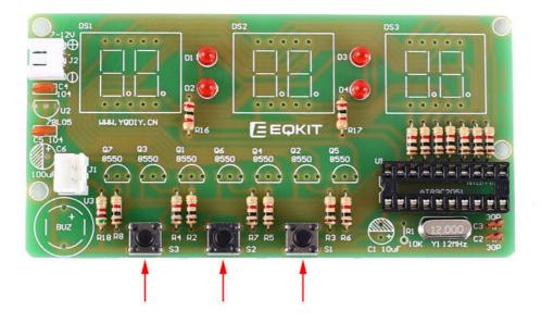
Step 12:Install 1pcs 10K Metal Film Resistor at R1.
